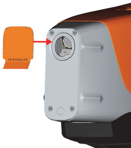
Figure 4-8 New window aligned with probe
